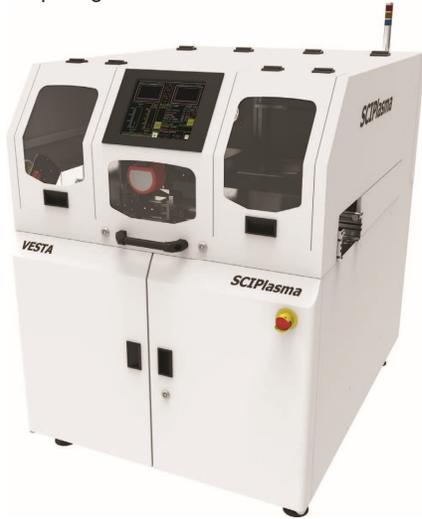
bondability of that specific assembly. Removing organic contamination or oxides left behind by previous process steps like die attach or snap curing are an easy task for a good plasma cleaning system. The [wire bond pull and shear forces](#) will increase, creating a much more reliable bond improving the overall bonding yield. An increased yield means a higher ROI for that particular product – so much so that the investment for a plasma cleaner could amortize rapidly.
